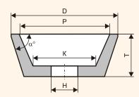
For flat grinding and spline-grinding the details and constructions made of cast iron, non-ferrous metals, natural and artificial stone, glass, porcelain, for hard-alloy cutting tools sharpening.
