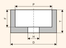
For flat, round inner grinding the details and constructions made of different types of steels, for sharpening the cutting tools made of high speed steels.
