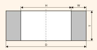
For flat grinding by a butt-end of the wheel of the details and constructions made of cast iron, non-ferrous metals and mineral materials.
