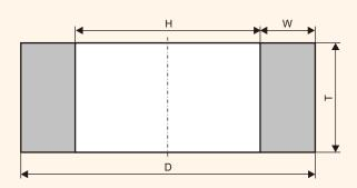
For flat grinding by a butt-end of the wheel of the details and constructions of different types of steels and also for the sharpening the cutting tools of high speed steels.
