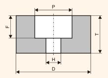
For all types of grinding operations the details and constructions made of cast iron, non-ferrous metals, natural and artificial stone, glass, porcelain, for sharpening the solid-alloy cutting tools.
