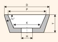
For flat grinding the details and constructions made of different kinds of steels, for spline-grinding, for cutting tools sharpening made from high speed steels
