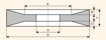
For all kinds of grinding with possibility of synchronous processing by a butt-end and a peripheral side of the details and constructions made of different types of steels, for sharpening the cutting tools made of high speed steels.
