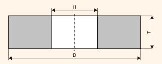
For flat grinding by a butt-end of the details and constructions made of different types of steels, sharpening of the cutting tools of high speed steels.
