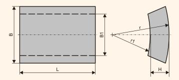
For flat grinding of the details and constructions made of different types of steels.
